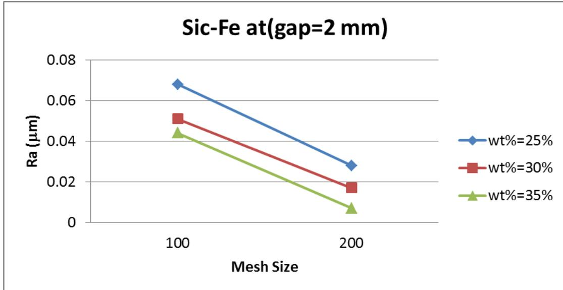
Figure (7) Relationship between mesh size and surface roughness at gap 2mm
