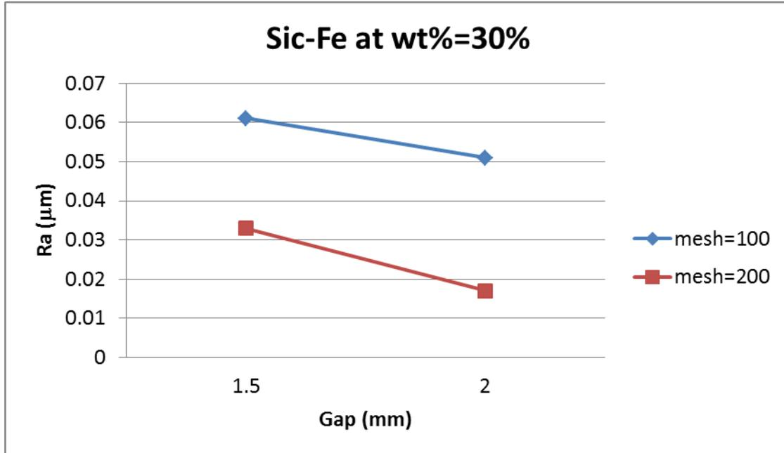
Figure (9) Relationship between gap size and surface roughness at 30%Si
