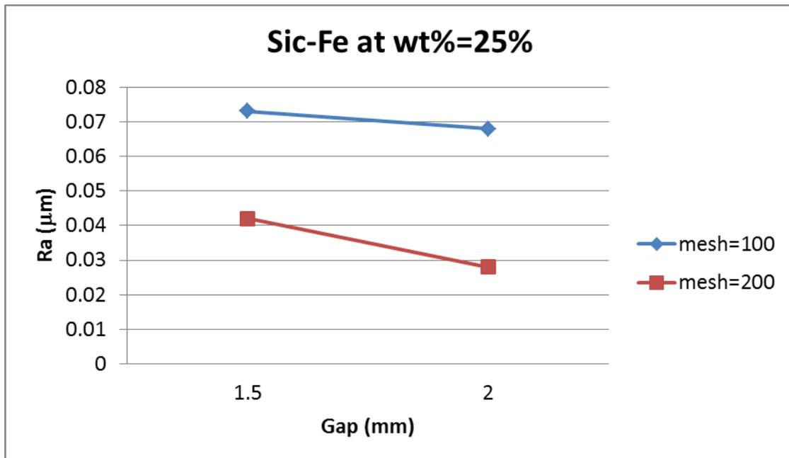
Figure (8) Relationship between gap size and surface roughness at 25% Si
