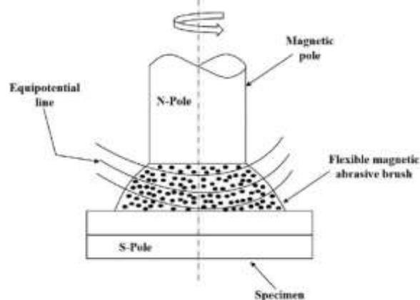
*Figure (1) principle of MAF process [2]*
