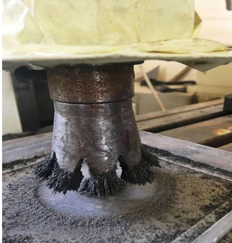
*Figure (5) machine of MAF process*
