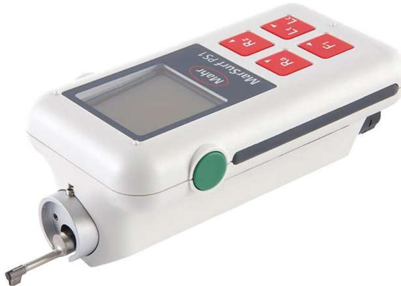
*Figure (19) surface roughness device*
