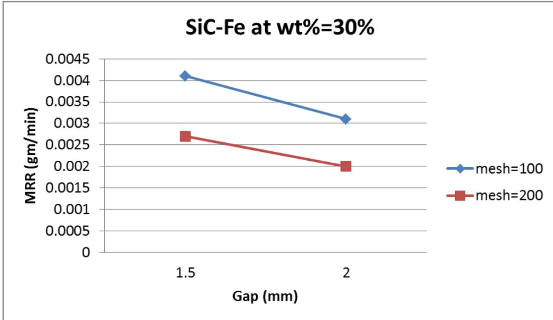
Figure (17) Relationship between gap size and metal removal rate at concentration 30% Si
