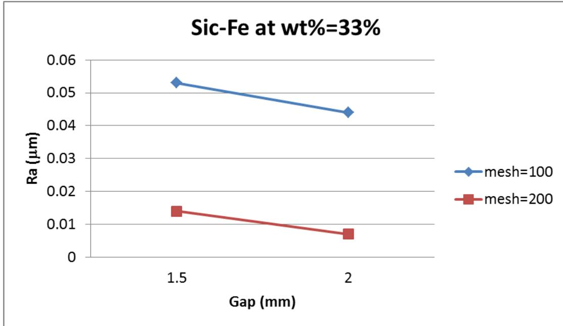
Figure (13) Relationship between mesh size and surface roughness at concentration 33% Si
