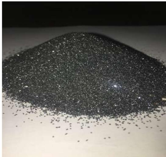
Figure (3) Abrasive of silicon carbide
