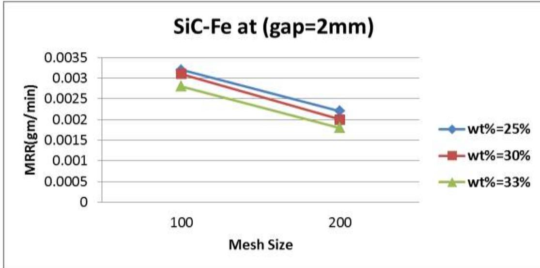
Figure (15) Relationship between mesh size and metal removal rate at gap 2mm
