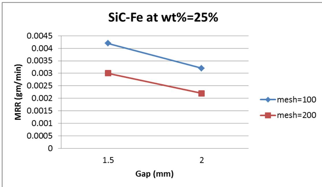
Figure (16) Relationship between gap size and metal removal rate at concentration 25% Si
